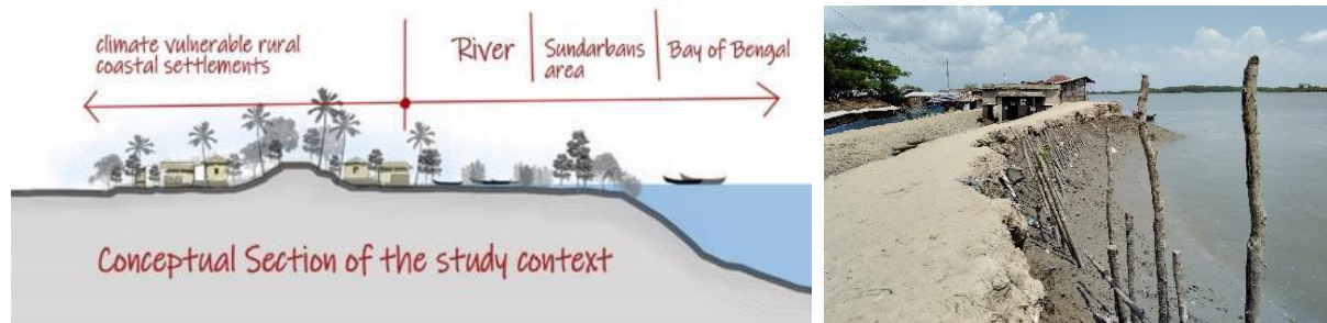
Figure 2. Conceptual drawing of the study area (left) and the embankment vulnerability (right)
