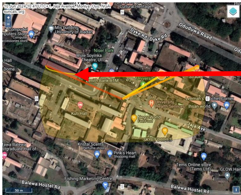
Plate 2: Sun Path diagram of the study location
