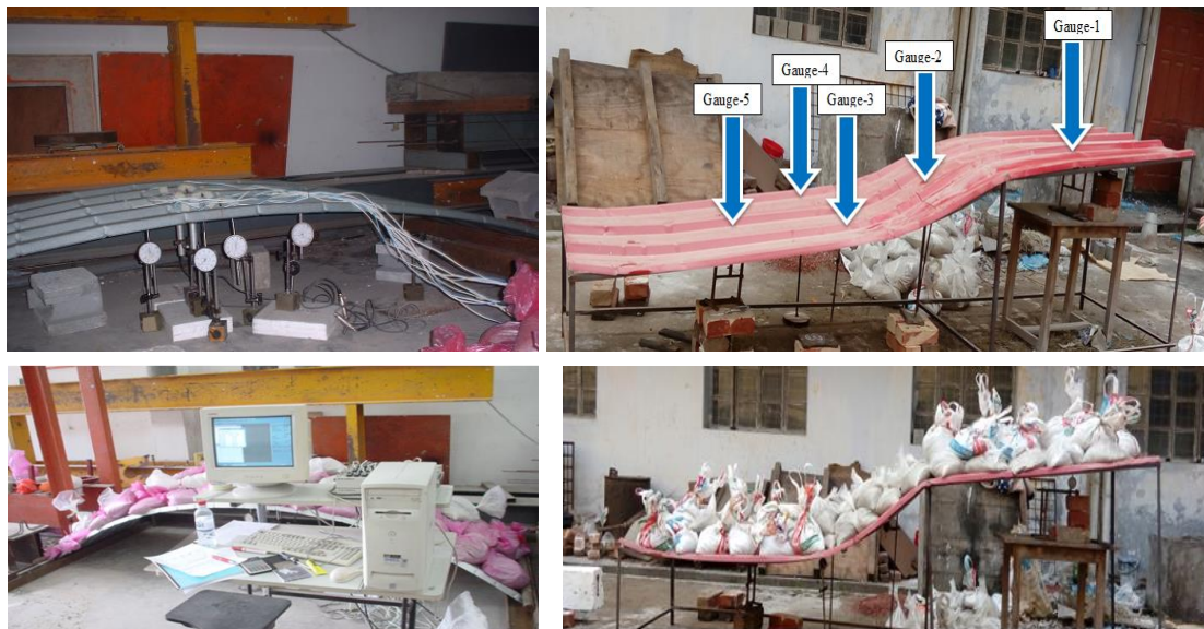
Figure 4. Test setup and sand bag loading on parabolic and doubly curved of roofing element.
