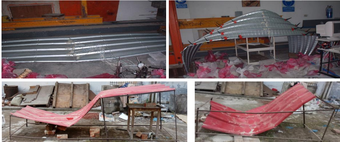
Figure 5. Failure mode of parabolic and doubly curved of roofing element.
