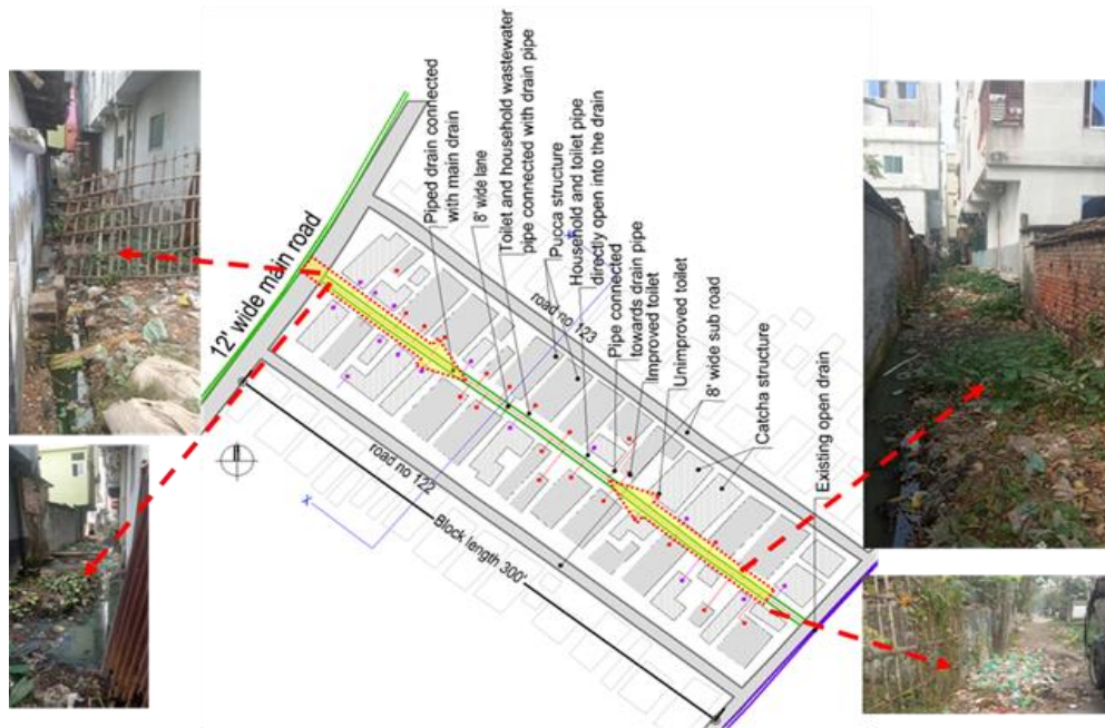
Figure 8. Housing map between roads 122 and 123 (sample block) with a piped drainage system. (Source: author)
